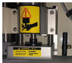
钨钢铣刀+刻字刀 Multi-function cutting head
