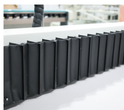
风琴护罩 Organ-like dust shield
