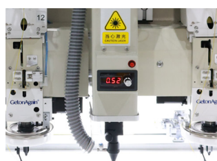
(选配) 激光切割装置 (Optional) laser cutting device
